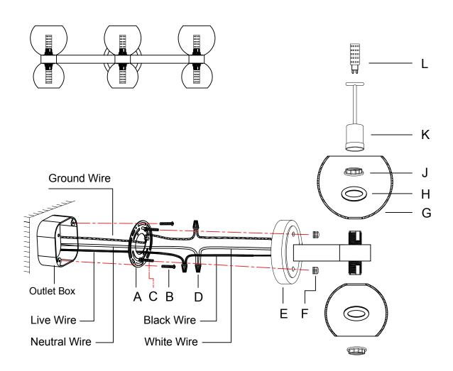
In view of thermal expansion and contraction, avoid securing the glass shade too tight when screwing the socket ring into the lamp holder, otherwise you may break the glass shade.
