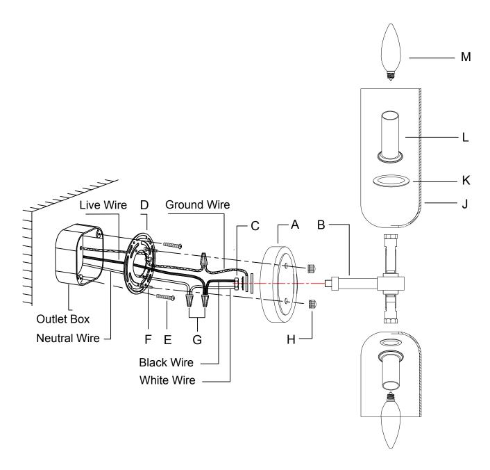
In view of thermal expansion and contraction, avoid securing the glass shade too tight when screwing the socket ring into the lamp holder, or you will break the glass shade.
