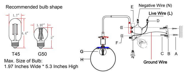
Note: The way to differ the negative wire from the live wire is that a white line is printed on the cover of the negative wire.
