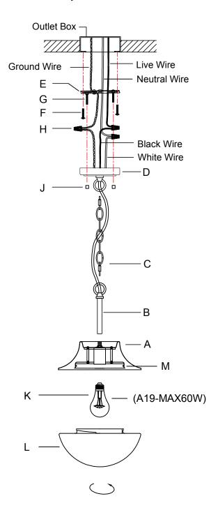
You can turn the pendant light into a semi flush-mount ceiling light by removing the ring attached to the canopy and the hanging rod and screwing the canopy into the hanging rod.
